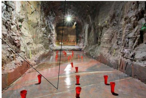
Fig. 10. Test site at Äspö HRL after diamond wire cutting (Photo: Rickard Enér)
